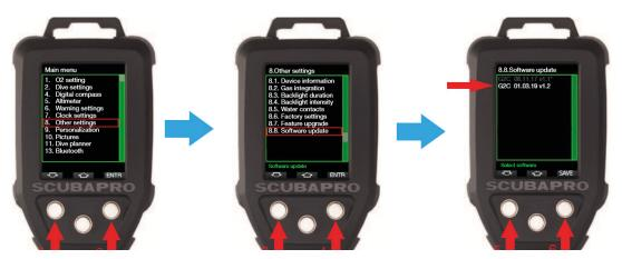
Repeat until you reach "8.8 Software update". Press the right button, choose the latest Software and save your changes by pressing the right button again. The Software currently installed on your G2 is marked by an asterix [\*].
