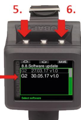
Repeat until you reach "8.8 Software update". Press the right button, choose the latest Software and save your changes by pressing the right button again. The Software currently installed on your G2 is marked by an asterix [\*].
