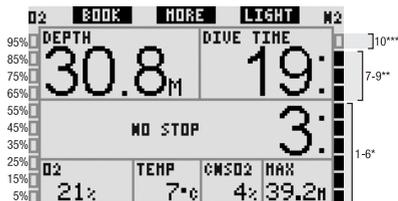
**Nitrogen bar graph:** This is the bar graph on the right side of the display (**CLASSIC**, **LIGHT** and **FULL** configurations). It represents nitrogen saturation in the leading tissue compartment. The bar graph is made of ten segments. The first nine segments represent gradually more loading but still within no-stop diving; the tenth segment represents the need for a mandatory decompression stop.
